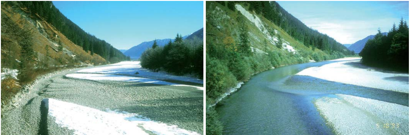
Ensuring ecological flow at the upper stretch of the river „Isar“ in Germany. The pictures show the river before and after measures for ensuring ecological flow requirements were implemented. Water flow which was previously completely diverted to “Walchensee” is now permanently provided through the river to “Sylvenstein” reservoir, also including some seasonal variations.
